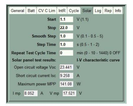
Enter the **Start** test voltage. Usually 1.1V to allow for the panel short circuit current measurement. KP184 minimum load voltage is about 1V.
