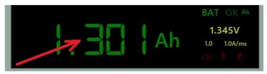
Clicking the battery capacity value large indicator resets its value. This can only be done with the load off to avoid inadvertently resetting it during the test.
