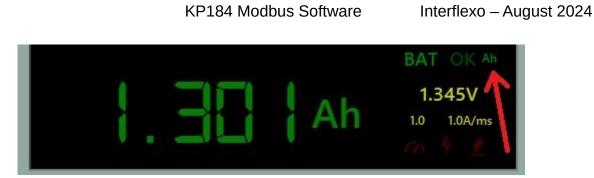
Clicking the Ah/Wh small indicator toggles the battery capacity value large indicator units between Ah and Wh.
